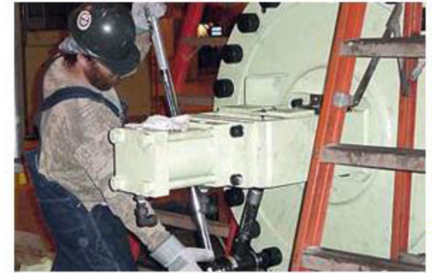
Torque bolts on injection mold machine
