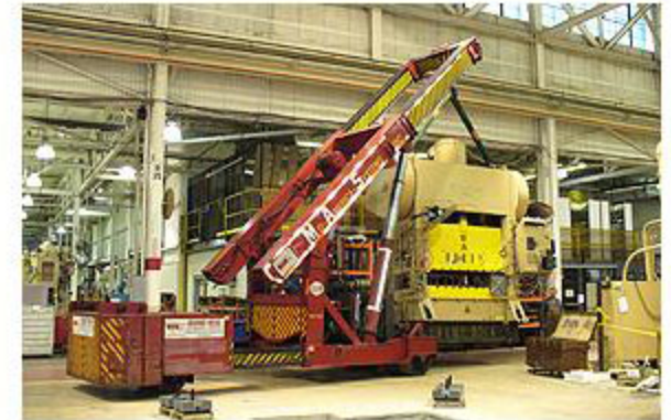
50 ton twinlift moving a machine
