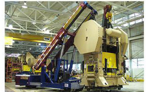
50 ton twinlift and 50 ton mobilift relocating a press in plant move
