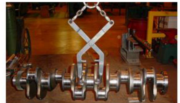
Lifting device made by MAS industrial blacksmiths
