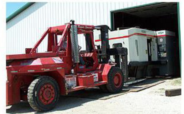
40/60/80 riggers special moving a machine into a building
