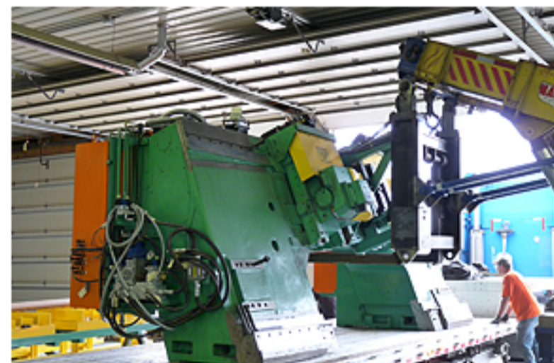
34 ton twinlift with fork attachment unloading a machine sitting flat on truck floor
