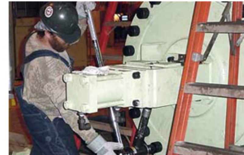
Torque bolts on injection mold machine
